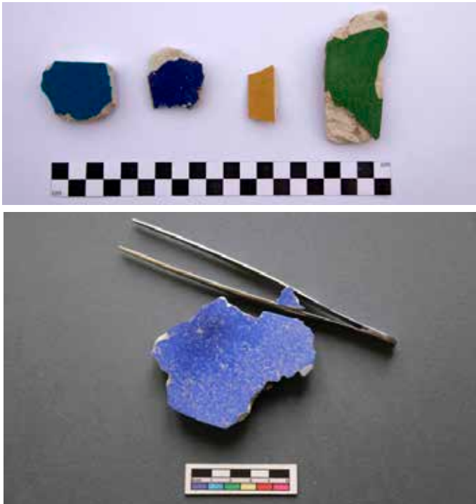
Tile samples were tested and replicated to match the original in composition and colour
