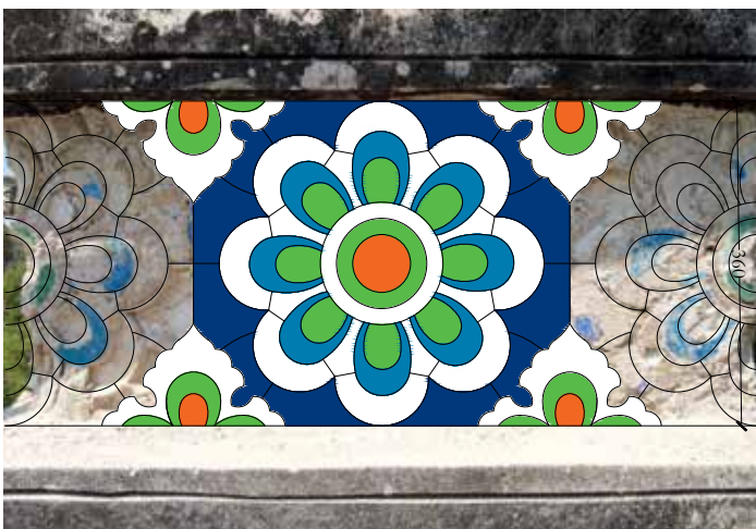
Master craftspeople carefully cut each tile to shape and size, creating samples of the motifs based on the formwork and scaled drawing, ensuring they match the original details revealed
